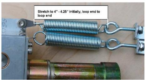
Figure 7 Spring initial tension setting for bracket placement
