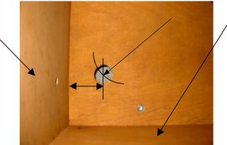
Figure 3 Inside of rocker showing roller hole placement
