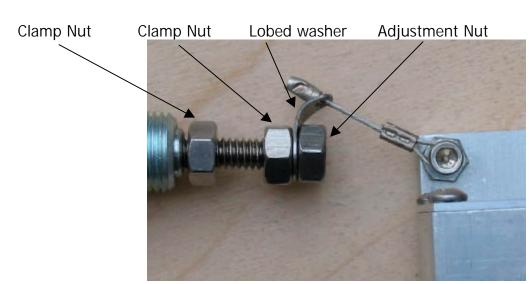
Figure 6 AZ clamp adjust cable
