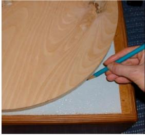
Figure 2 Radius mark from ground board edge
