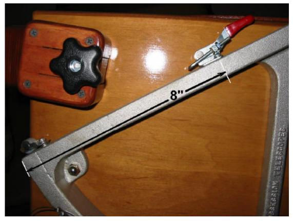
Fig 5c Clamp Mounting
