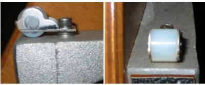
Fig 5b bearing roller placement
