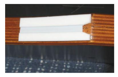
3) Locate the 2 supplied Teflon pads. These pads are ~3" long and 1" wide and have a groove milled down their length. Align each pad from just where the edge of the wood curve starts. Lift one pad at a time, run a bead of wood glue along the length of
